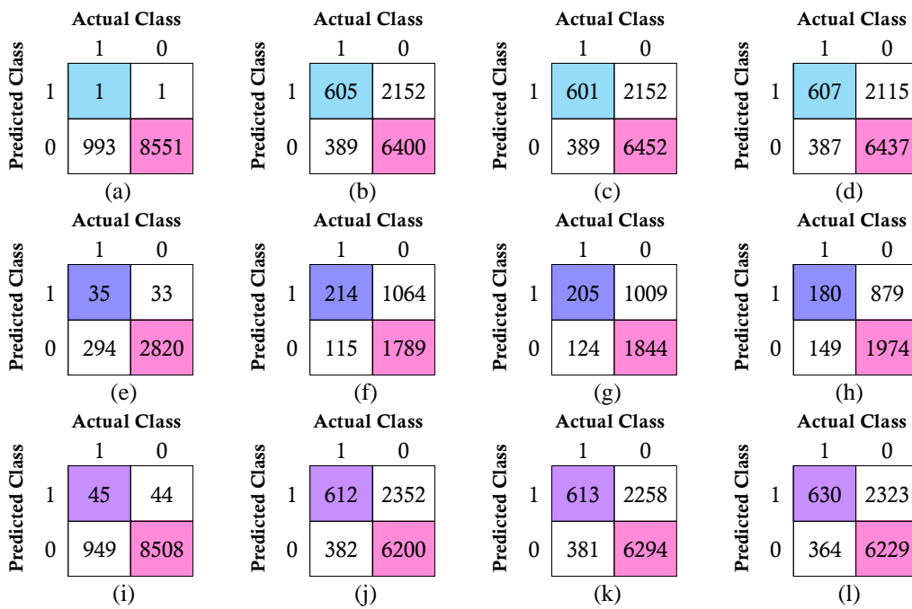
Figure 4 The confusion matrices across four different samplings in three classification models with train/test ratio of 70/30: (a) – (d) RF models; (e) – (h) KNN models; (i) – (l) XGB models.
