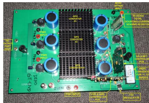
Figure 16 Photo of 3-channel DIPO converter power prototype showing three PCBs: one power PCB, and two controller PCBs
