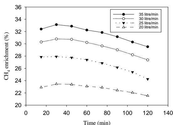
**Figure 7** Amount of  $\text{CH}_4$  recovery according to the testing time
