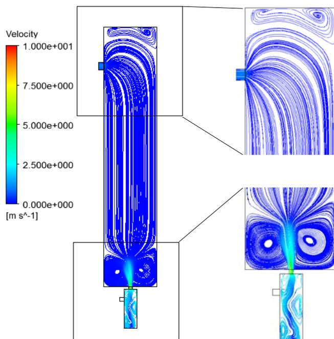
Figure 4 Velocity streamline at the center plane
