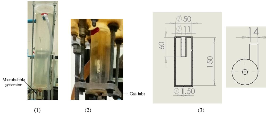
**Figure 2** Actual image of: (1) water column and (2) microbubble generator and (3) details of microbubble generator
