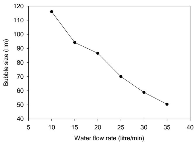
**Figure 6** Bubble size of each water flow rate
