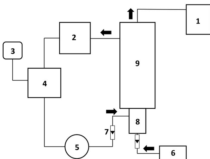
**Figure 1** Flow circuit (blue: water, orange: gas) and experimental apparatus of biogas upgrading pilot scale: (1) biogas analyzer, (2) cooling unit, (3) temperature control unit, (4) heater chamber, (5) pump, (6) raw biogas container, (7) gas flow meter, (8) microbubble generator and (9) reactor
