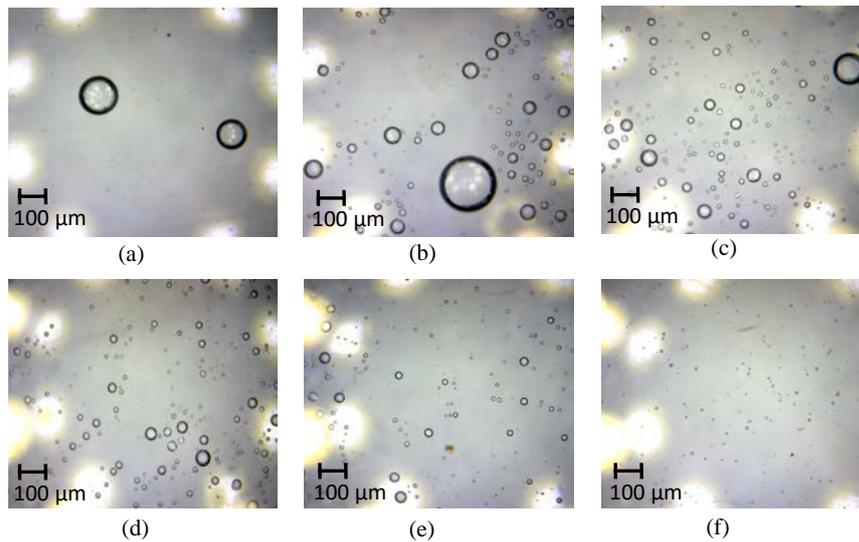
**Figure 5** Sampling bubble from microscope camera in cases of water flow rate (a) 10 litre/min, (b) 15 litre/min, (c) 20 litre/min, (d) 25 litre/min, (e) 30 litre/min, (f) 35 litre/min.
