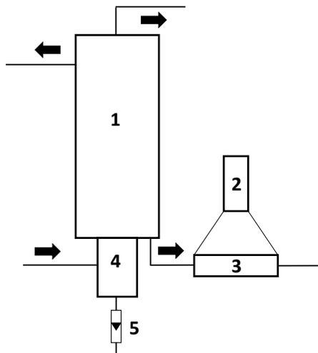
**Figure 3** Experiment setup for bubble size measurement (1) Water column, (2) microscope camera, (3) glass chamber, (4) microbubble generator and (5) flow meter
