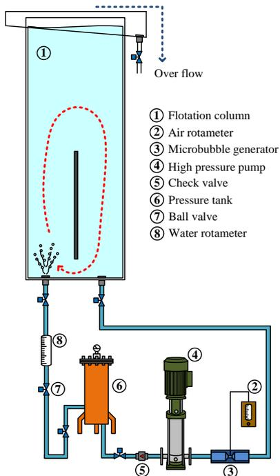
Figure 2 Experimental setup
