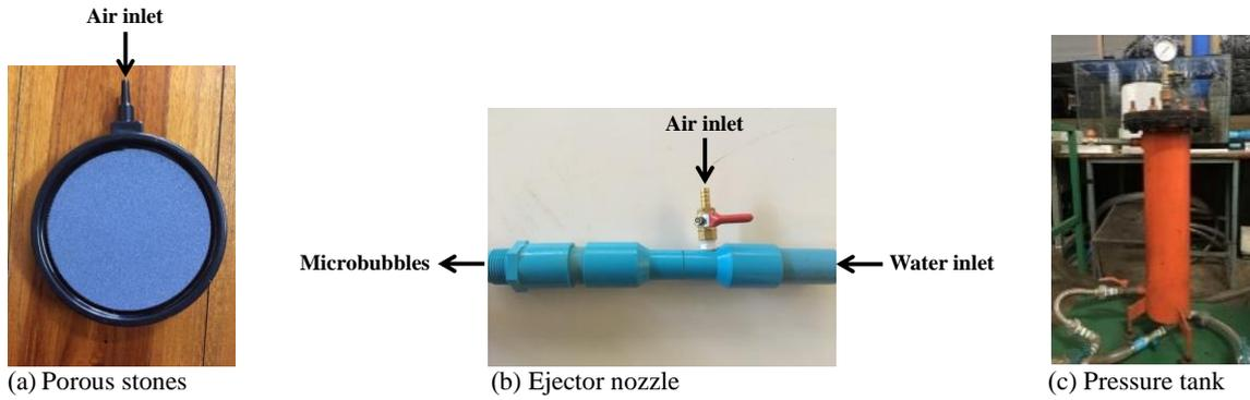
Figure 1 Microbubble generators
