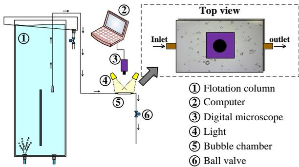
Figure 3 Experimental apparatus for the measurement of bubble diameter
