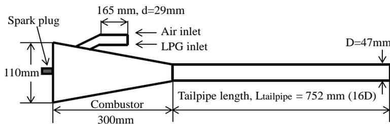
**Figure 3** Schematic diagram of a Helmholtz-type pulse combustor
