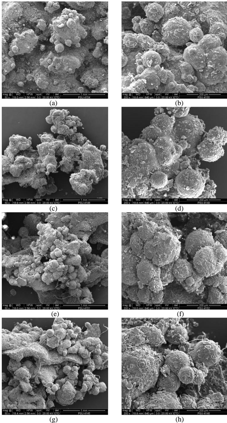
**Figure 9** The SEM micrographs for the natural rubber (NR) particles at different magnifications containing:
