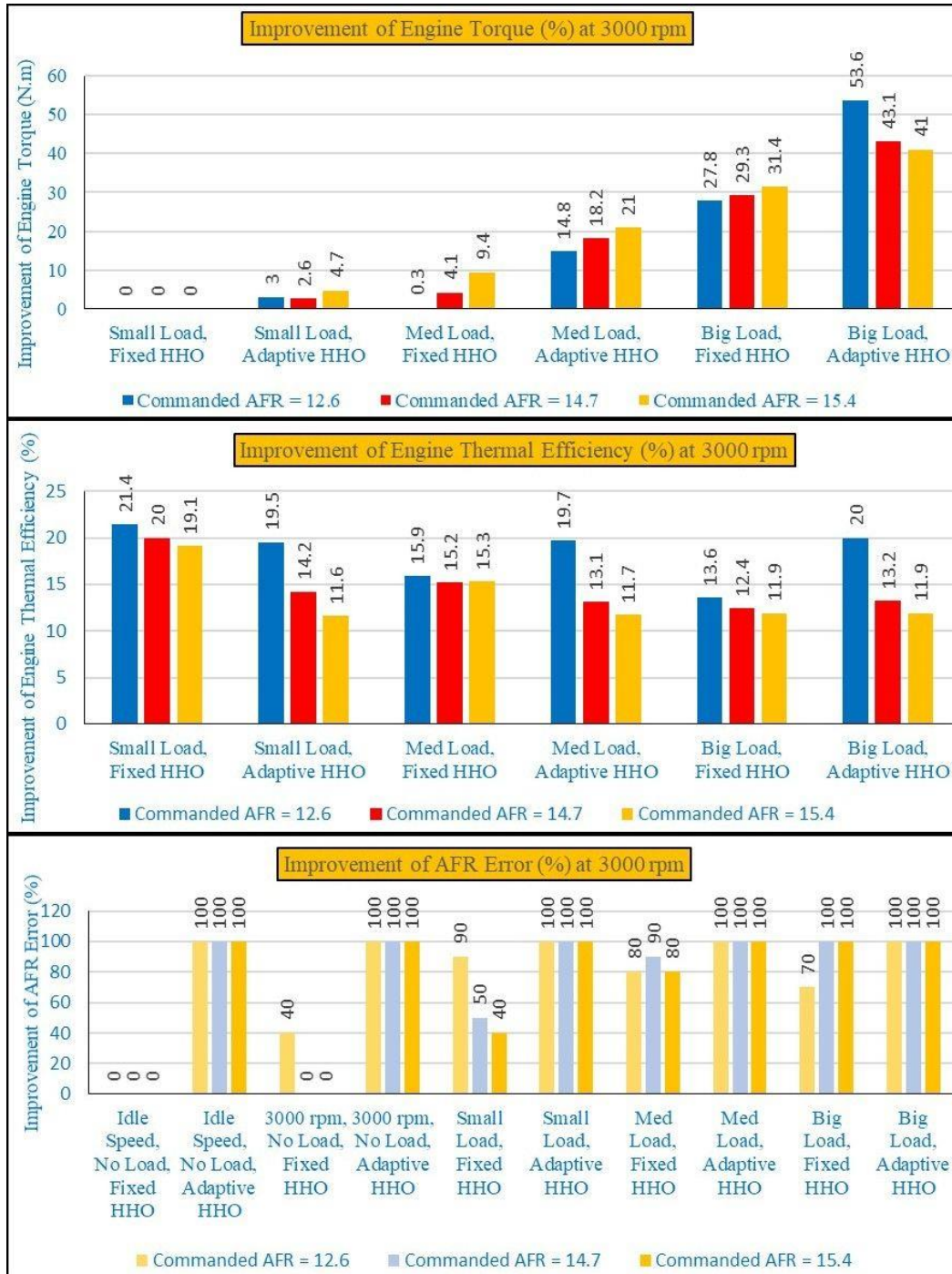
Figure 13 Improvement comparison of gasoline engine performance using the fixed and adaptive HHO flow rates at 3000 rpm, various loads and commanded AFRs
