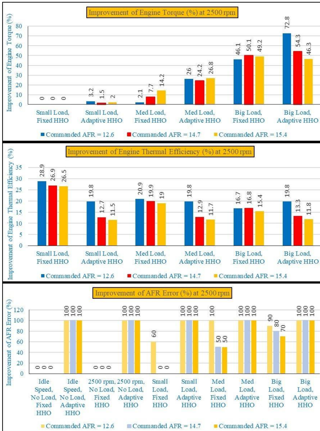
Figure 12 Improvement comparison of gasoline engine performance using the fixed and adaptive HHO flow rates at 2500 rpm, various loads and commanded AFRs
