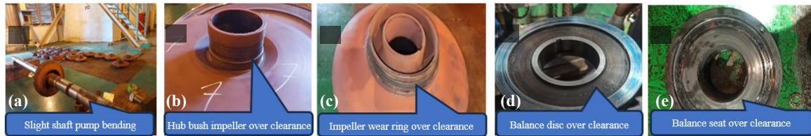
Figure 18 Field inspection results of boiler feed pump components following the LSTM-AE-based anomaly detection: (a) slight shaft pump bending, (b) hub bush impeller over clearance, (c) impeller wear ring over clearance, (d) balance disc over clearance, and (e) balance seat over clearance
