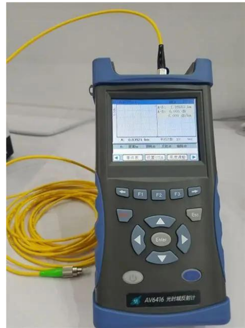
Figure 5 OTDR for measuring fiber optic performance
