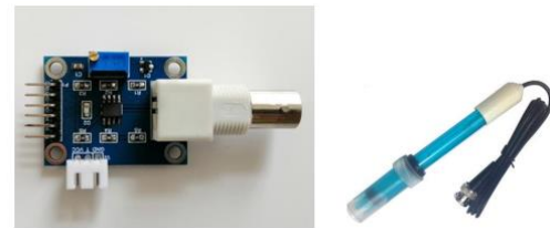
Figure 6 Schematic diagram of pH sensor module [12]
