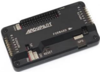
Fig. 2. APM 2.8 Flight Controller [6]
